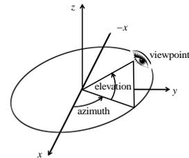
Fig. 3. The illustration of how we get the projections of a 3D shape model  $S$ . Azimuth is the polar angle in the  $x$ - $y$  plane, with positive number indicating anticlockwise rotation of the viewpoint. As for elevation, positive and negative numbers are the angle above and below the  $x$ - $y$  plane respectively.
