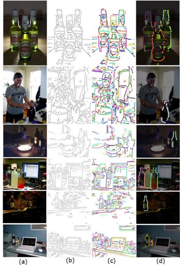
Figure 2. Bottles detection results when edges are severely broken. (a) shows bottle images from PASCAL dataset [7]; (b) shows the edge maps computed using Pb edge detector [18]; (c) shows edge-linking results by [13]; (d) shows our bottle detection results using a bottle FSM trained on ETHZ dataset [11] (shown in Fig. 5).
